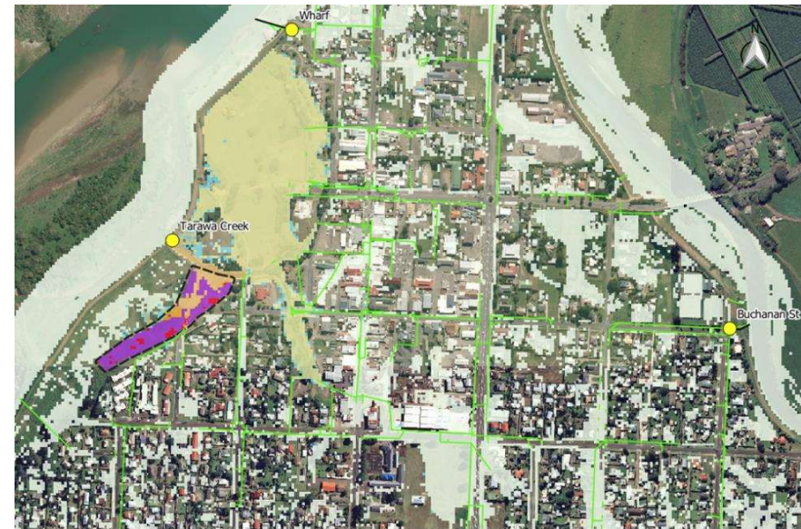
Figure 11-10 : Areas of surface flooding in Ōpōtiki Township for 10% AEP
