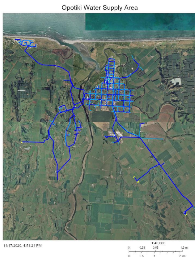
Figure 3-4 Ōpōtiki Township water supply network
